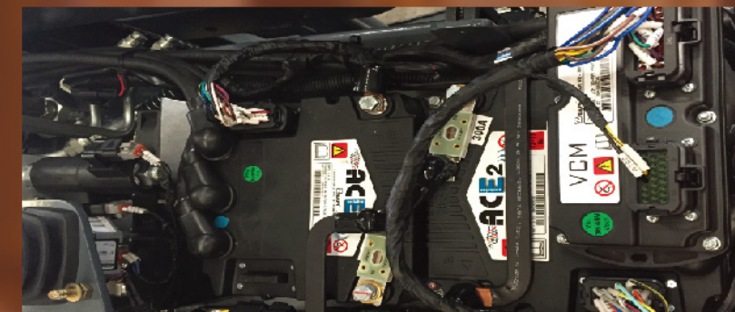
Easy to remove covers to access all electric and hydraulic components
